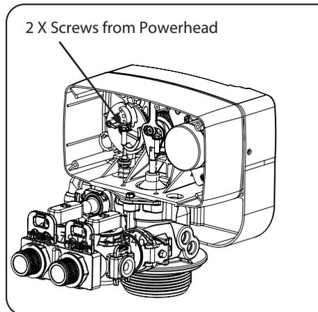
4. Remove the two screws from the powerhead as shown
