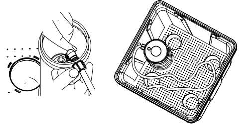
b) Insert the brine well assembly inside the grid plate as shown below.
