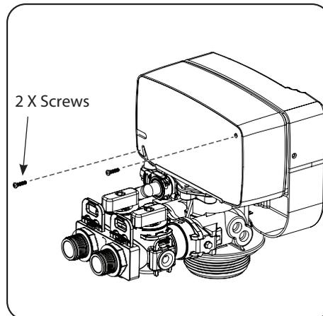
2. Remove two screws from the back of the valve cover
