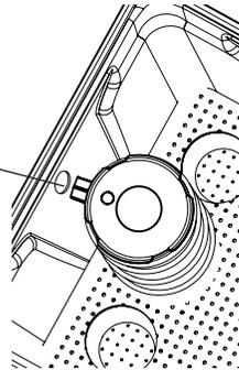
f) For installation of brine tank at the installation site, pull the other end of the brine tube from the hole on the brine tank. The completed assembly is shown on right.
