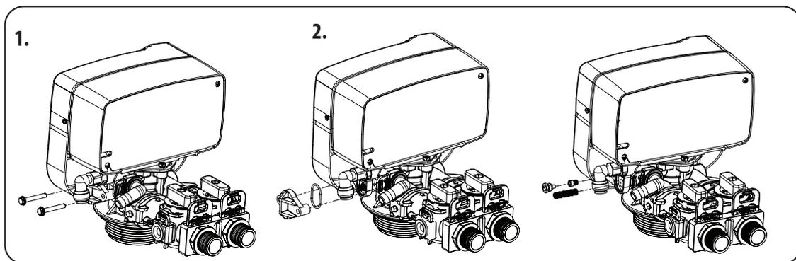
1. Remove two screws of the injector cap.
