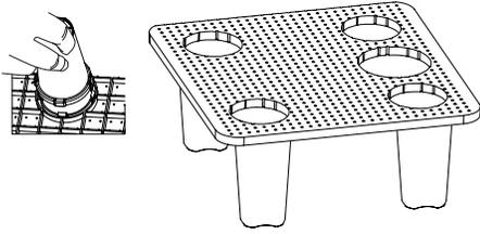
c) Drop the brine grid with brine well inside the brine tank such that the nut fitting faces the hole on the brine tank. Then press the grid evenly inside the brine tank until the brine grid legs touches the bottom of the brine tank.
