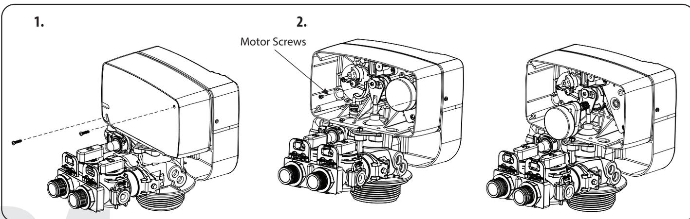
1. Remove back cover by removing two screws
