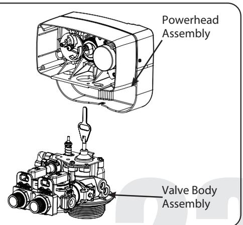
6. Replace the powerhead by reverse following the steps in this section
