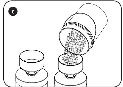
**c)** Fill support bed first. The media will not always spill down inside the tank and may need to be swept inside. The large funnel (sold separately makes filling the tank easier and neater. (Or an empty 1 gallon or 4 liter container with the bottom cut out makes a good funnel.)
