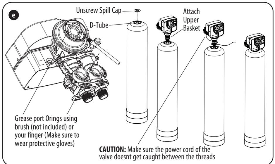
**d)** Lube the bottom Valve Orings with the grease supplied, Attach the Upper Basket. Unscrew the spill cap. Carefully Slide the D-Tube inside the Valve and Screw the Valve inside the Tank such that the power cord doesn't get caught between the valve and the tank.
