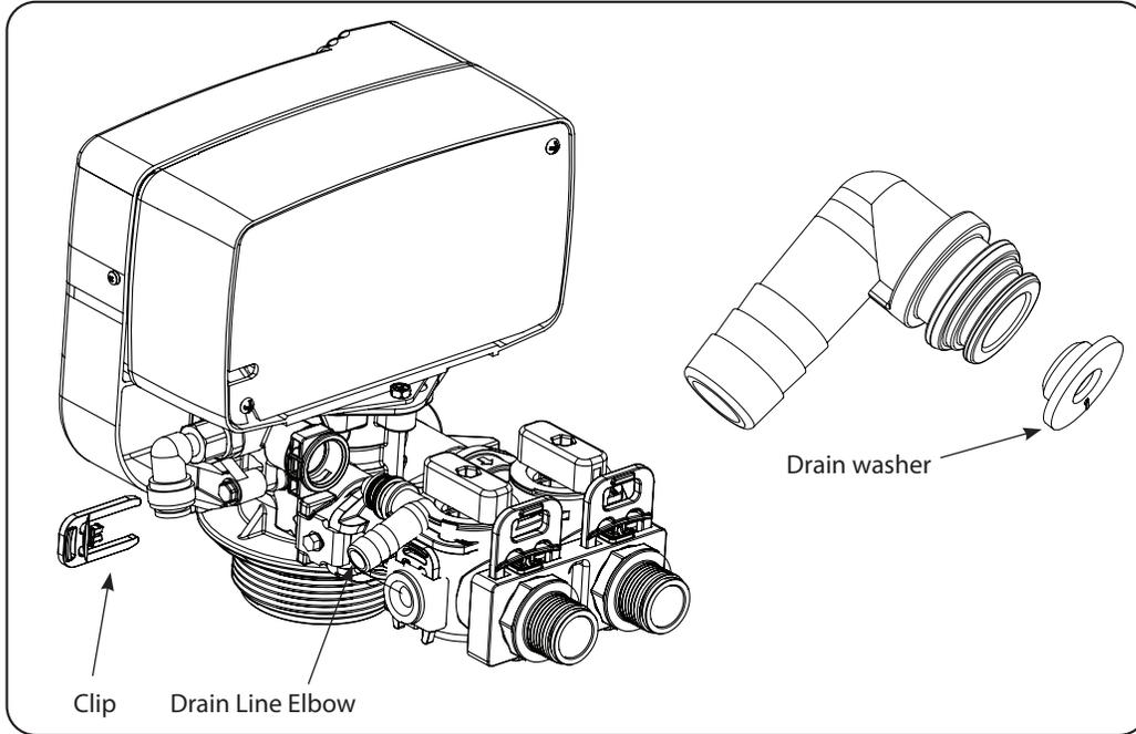
1. Pull the drain line clip and remove the drain line elbow and washer
