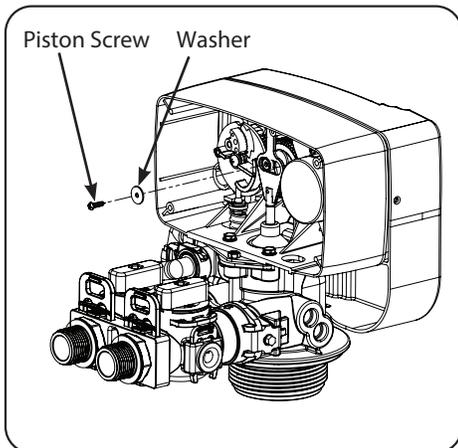
3. Remove the piston screw and washer from the piston rod.
