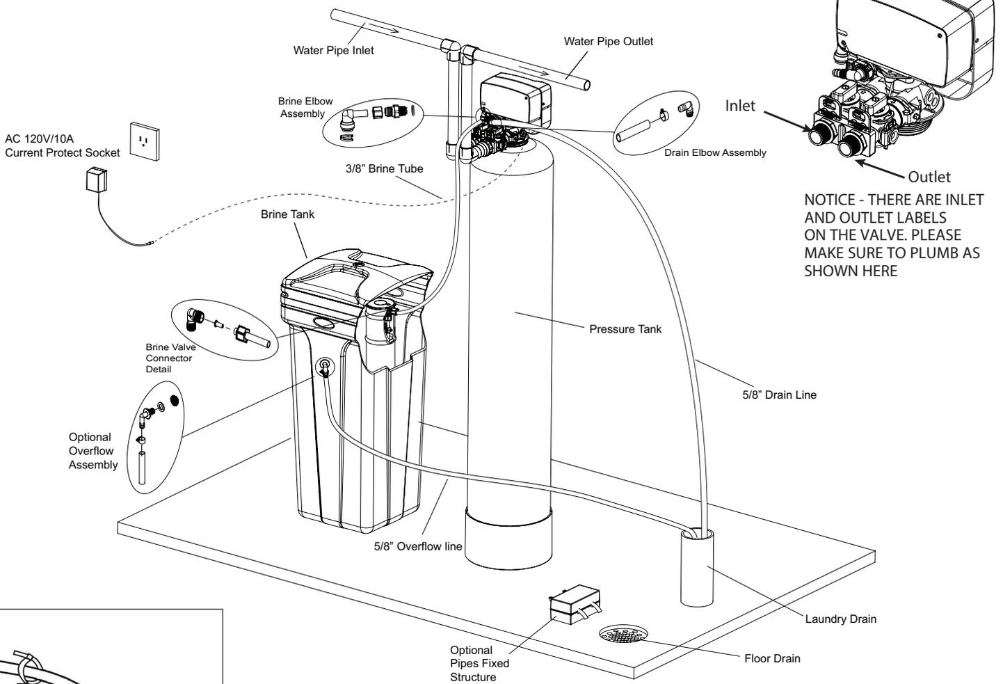
NOTICE - THERE ARE INLET AND OUTLET LABELS ON THE VALVE. PLEASE MAKE SURE TO PLUMB AS SHOWN HERE
