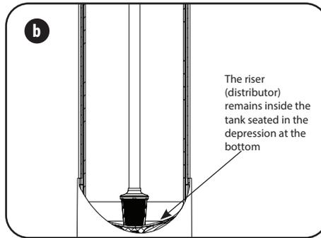
**b)** Temporarily plug the open end of the riser tube to ensure that no resin or gravel falls down into the distribution. The riser (distributor) remains inside the tank seated in the depression at the bottom. Plug tube with a tape. Remove after media is loaded.
