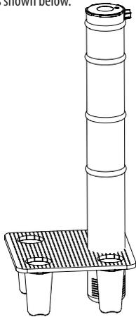
IMPORTANT: The hole in the brine tank should line up with the brine line as shown.
