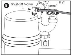
5. Attach Tubing to Tank Shut-off Valve
