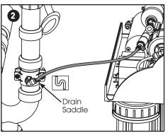
2. Attach the other end of the 1/4" tubing to the drain saddle
