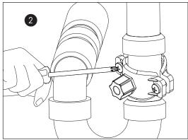
2. Tighten the clamps with the help of the two bolts.
