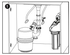
Place Tank under the sink. The Shut off valve is already installed in the early steps
