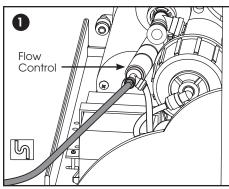
Attach 1/4" Tubing to Flow Control
