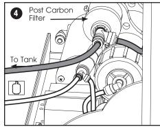
**4.** Attach 3/8" Tubing to Post Carbon Filter
