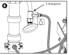
8. Connect Tubing from T-Adaptor to RO Inlet
