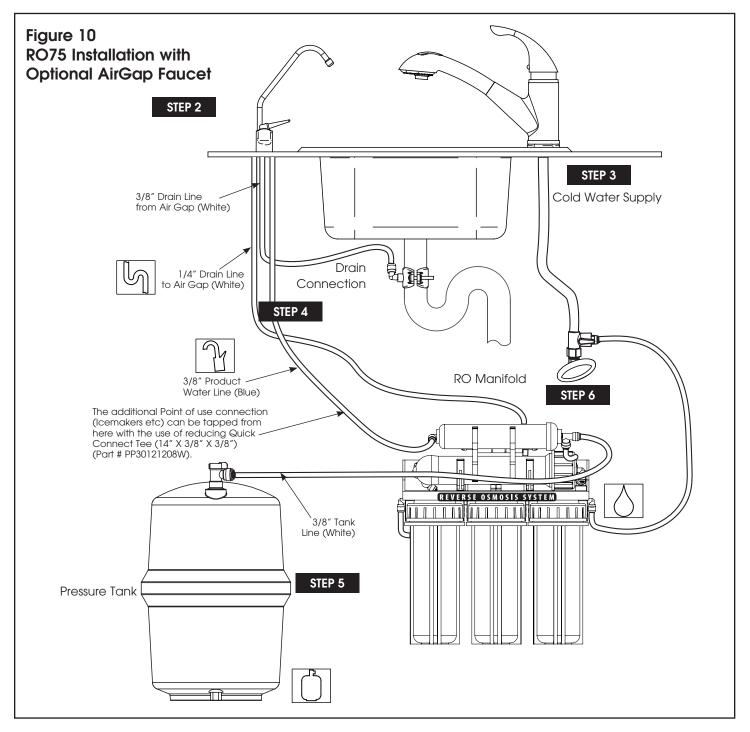
**NOTE:** Install the 3/8" red drain line from the air gap faucet to the drain adapter so that it runs downward with no loops or low spots. Otherwise the unit will overflow at the air gap siphon break built into the faucet, or make irritating gurgling sounds.
