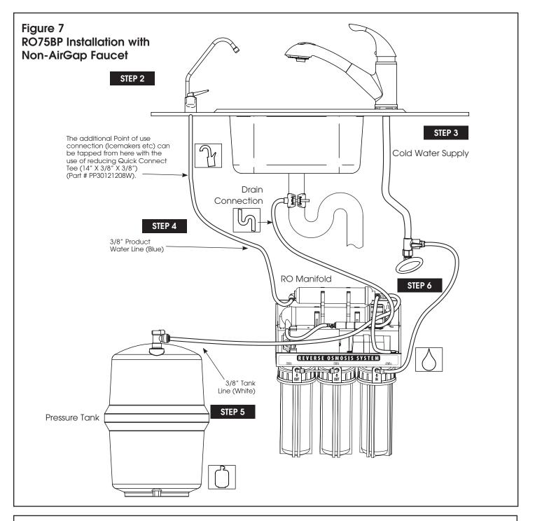
**NOTE:** Install the 3/8" red drain line from the air gap faucet to the drain adapter so that it runs downward with no loops or low spots. Otherwise the unit will overflow at the air gap siphon break built into the faucet, or make irritating gurgling sounds.
