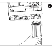
7. Attach Sump to Manifold
