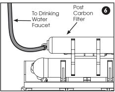
6. Attach Tubing to Post Carbon Filter
