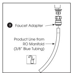
3. Take another length of 3/8" tubing and make sure it is has a fresh cut and is free of foreign materials and any scratches on the outside surface. Install the tubing into the push in type fitting at the base of the faucet. Make certain that it is inserted all the way in; once inserted give it a slight pull to make sure it is locked into the fitting. You have now completed the tubing connections.
