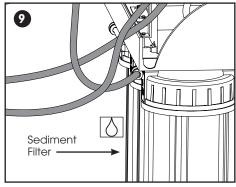
9. Connect Tubing from T-Adaptor to RO Inlet
